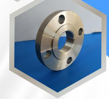
Threaded Flanges provide a secure connection without welding, ideal for high-pressure piping with low-temperature operations. Manufactured from carbon/alloy steel with IBR and non-IBR variants. Sizes: ½" to 12", pressure: Class 150–600. Standards: ASME B16.5, IS 6392. Commonly used in gas lines, fire protection and boiler piping systems where welding is not feasible.
