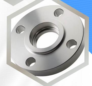
Slip On Flanges are designed to slip over pipe ends for easy alignment and welding. Available in IBR and non-IBR certified carbon and alloy steel, sizes: 1/2" to 24", pressure ratings: Class 150 to 2500. Standards: ASME B16.5, IS 6392, IBR approved. Used in process piping, boiler lines and water treatment plants for easy installation and long-term leak-proof performance.
