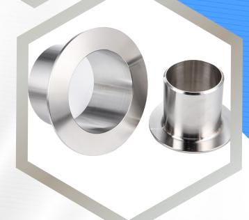
Short Stub Ends are used with lap joint flanges for easy disassembly. Available in IBR-certified and non-IBR carbon/alloy steel grades. Sizes: 1/2" to 24"; standards: ASME B16.9, MSS-SP-43. Widely used in pipelines requiring regular inspection or cleaning, especially in power plants, food and water systems.
