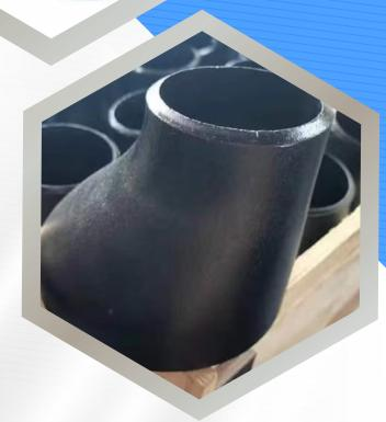
Eccentric Reducers provide offset flow transitions, often used at pump inlets to prevent air accumulation. Available in IBR and non-IBR carbon/alloy steel options. Sizes: ½" to 24", thickness: SCH 10 to XXS. Meets ASME B16.9 and IBR specifications. Installed in drainage, slurry transport and steam pipelines needing precise alignment and certified strength.
