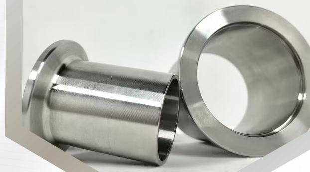
Long Stub Ends extend beyond the flange for alignment and rotation in piping. Made from IBR/non-IBR carbon steel, alloy steel. Sizes:  $\frac{1}{2}$ " to 24". Conforms to ASME B16.9 and IBR certification. Common in systems needing corrosion-resistant or regularly disassembled flanged joints, such as refineries and chemical plants.
