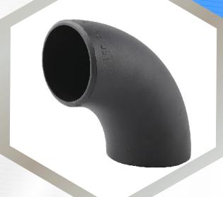
90° Steel Elbows change flow direction at a right angle, available in IBR and non-IBR categories. Materials: Carbon steel, Alloy steel; sizes: ½" to 24". Conforms to ASME B16.9 and IBR norms. Used in power plants, refineries and boiler lines where high-pressure, high-temperature performance is required with certified compliance.
