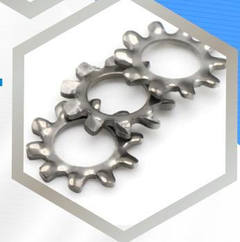
Star Washers have radial teeth and are ideal for applications requiring increased torque retention. Available in SS 304 and 316, sizes: M3 to M24. Compliant with DIN 6798. Used in electrical grounding, control systems, and electronics to provide secure, conductive connections and anti-vibration locking.
