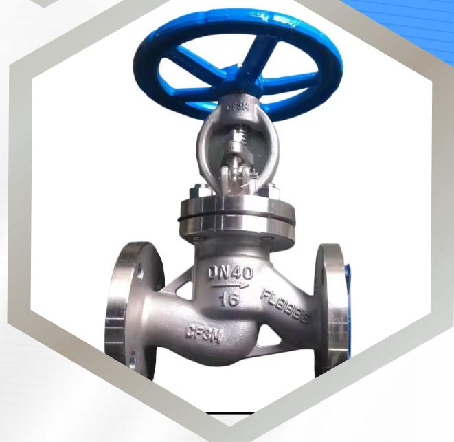
Globe Valves are used for regulating flow with a linear motion disc that opens and closes against the flow. Suitable for high-pressure and high-temperature applications. They provide excellent throttling capabilities. Made from SS 304, 316, and 316L, available in sizes  $\frac{1}{2}$ " to 12", with Class 150-1500 pressure ratings. Conforming to BS 1873, API 602, and ASME B16.34. These valves are ideal for steam, oil, gas and corrosive liquids in power, chemical and process industries.
