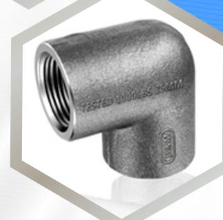
SS 90° Elbows are widely used to change pipe direction at a right angle, ensuring smooth flow transitions. Available in long and short radius types. They are manufactured from SS 304, 316, 316L, and 321 grades. Size range: 1/2" to 48"; Schedule: SCH 10 to SCH XXS. These elbows conform to ASME B16.9, ASTM A403 standards and are suitable for industries like oil & gas, chemical, water treatment and pharmaceuticals due to their strength and corrosion resistance.
