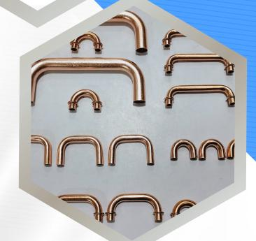
Copper C Bends are specialized fittings shaped like the letter 'C' to reroute pipelines while maintaining the same orientation. Made from deoxidized high-phosphorus copper (C12200), available in sizes from 1/4" to 2". Conforming to ASTM B75 and EN 1057 standards, these bends offer excellent ductility and resistance to dezincification and internal corrosion. Typically used in tight plumbing layouts, hot/cold water lines, and cooling systems where traditional elbows or tees cannot fit.
